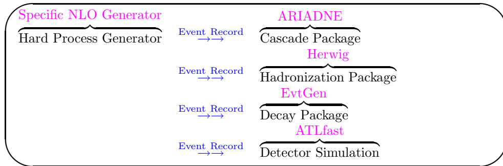
Figure 1: HepMC supports the concept of modularised event generation (illustrated above) by containing sufficient information within the event record to act as a messenger between two modular steps in the event generation process.
